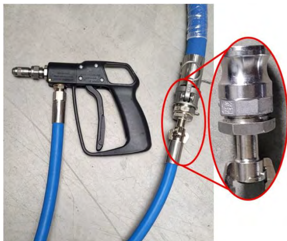
Figure 10: Adapter for hand spray gun
