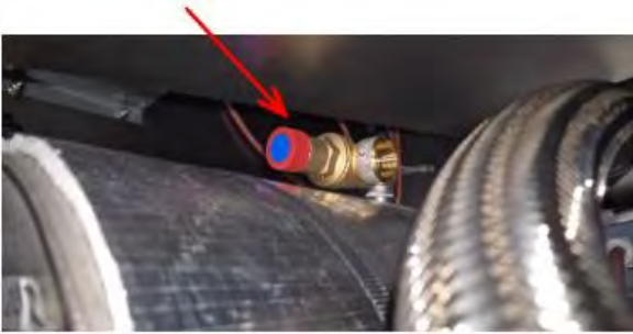
Figure 62: Heat Exchanger Safety Valve
