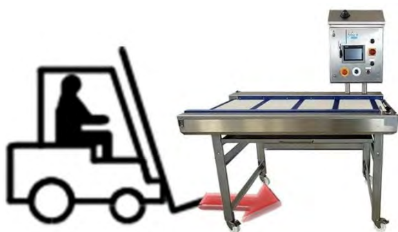
Figure 44: Lifting conveyor belts with a pallet jack or industrial truck
