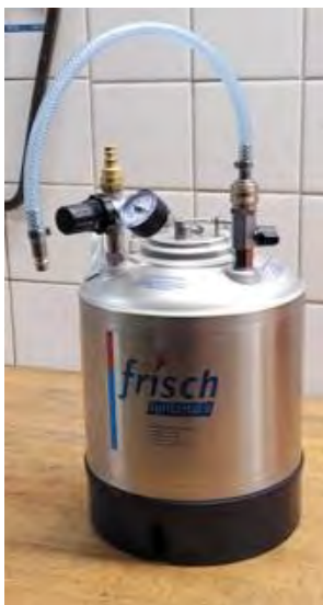
Figure 49: Example of a pressure tank
