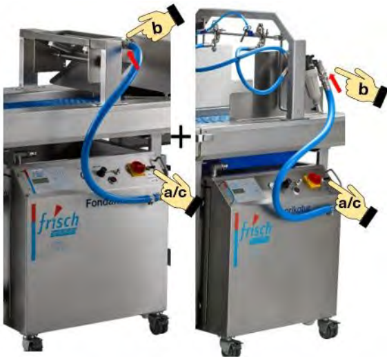
Figure 55: Connecting the Combino Jet to the conveyor system
