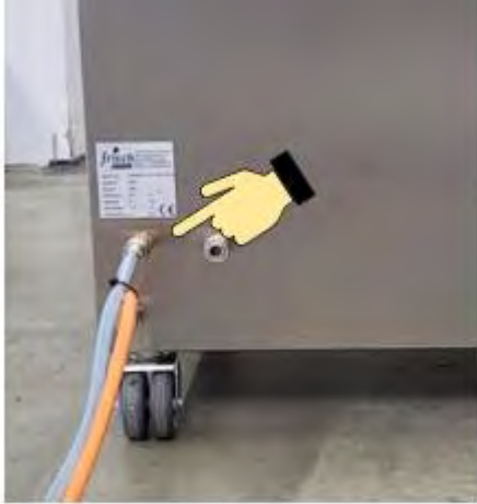
Figure 47: Establishing the compressed air supply
