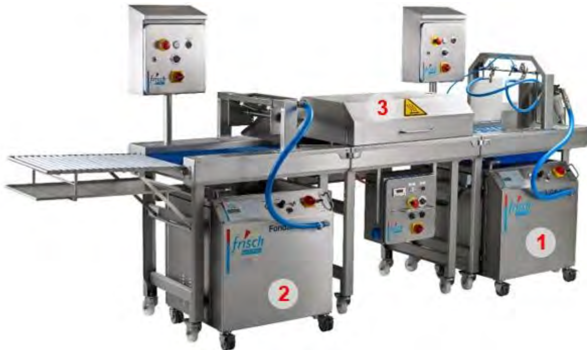
Figure 1: Example combination of heating machines and a Combino conveyor system
