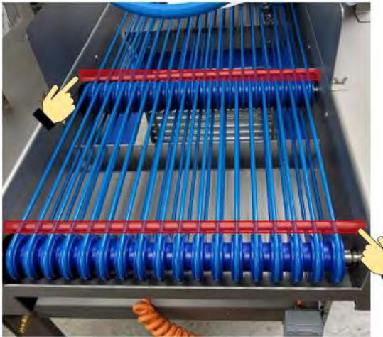
Figure 16: Filler pieces on the conveyor belt
