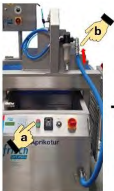
Figure 42: Filling the glazing station
