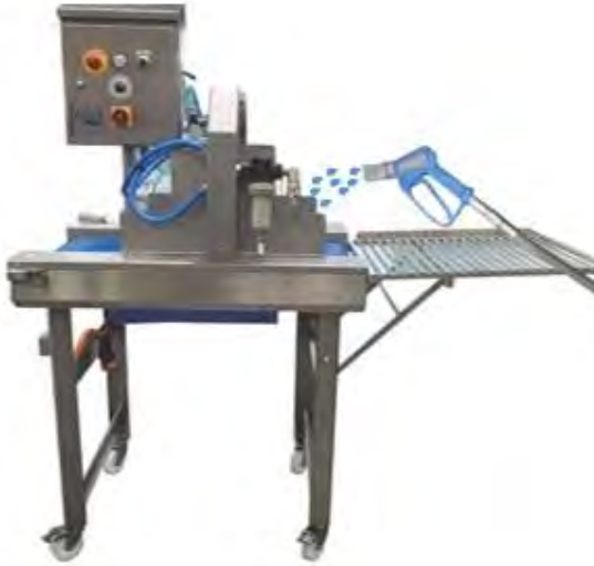
Figure 56: Cleaning the belt
