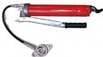
Figure 62: Lubricate with the grease gun
