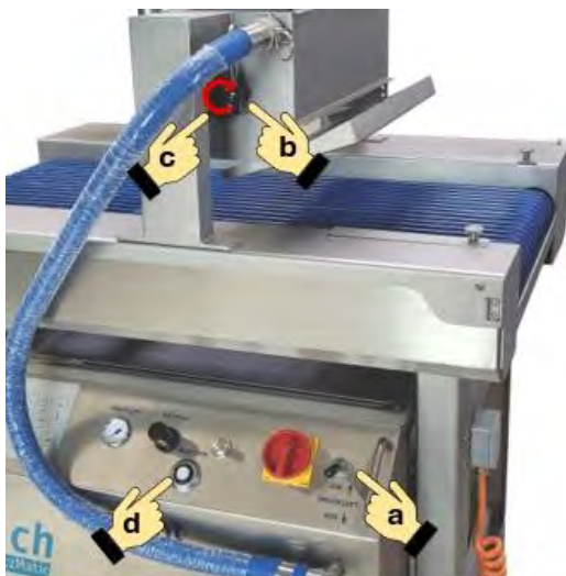
Figure 41: Filling the glazing station
