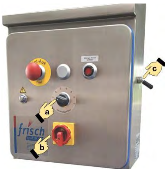
Figure 45: Switch off the main switch on the modules
