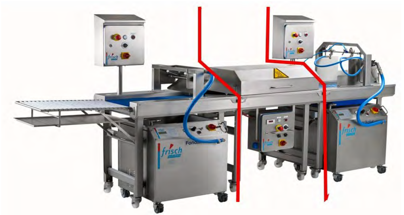
Figure 46: Positions of the module interfaces
