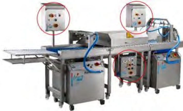
Figure 44: Positions of the control cabinets
