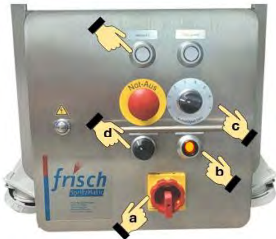
Figure 25: Switching on the heat tunnel
