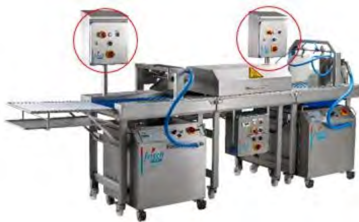
Figure 34: Positions of the control cabinets
