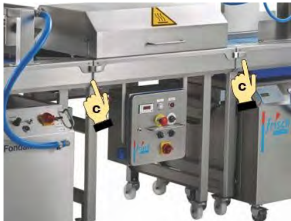
Figure 36: Locking quick-release clamps
