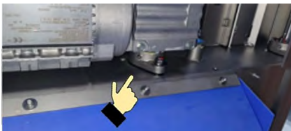
Figure 61: Bearing behind the drive motor
