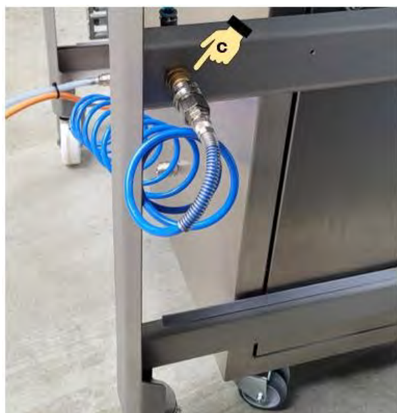
Figure 20: Establishing the compressed air supply Apricot belt
