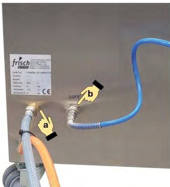
Figure 19: Establishing the compressed air supply
