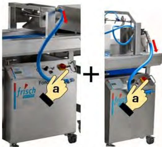
Figure 47: Unlocking the quick-release clamp
