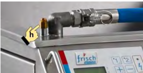
Figure 69: Pressure relief valve
