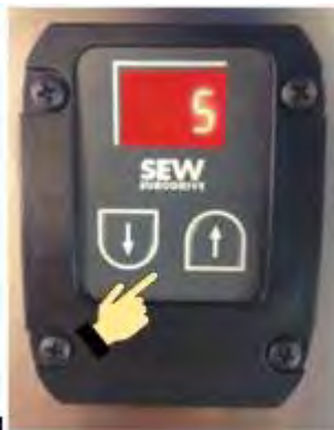
Figure 54: Controlling pump speed
