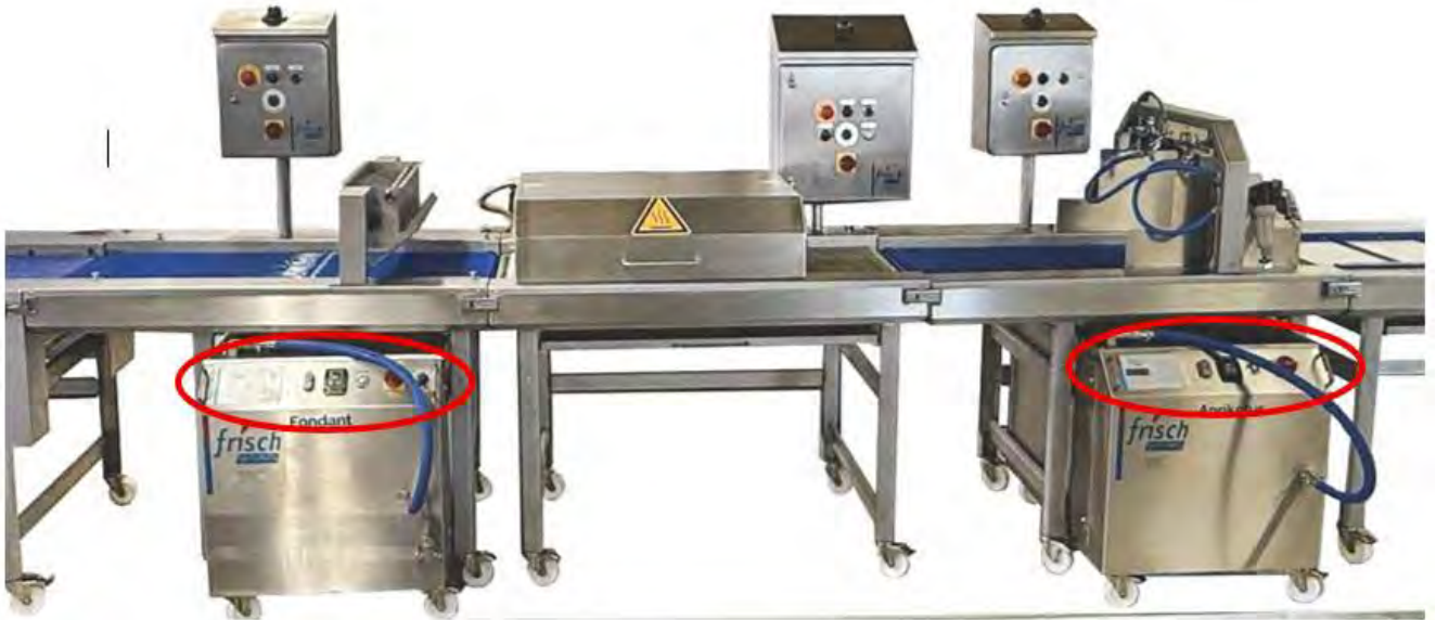
Figure 43: Heating machine position
