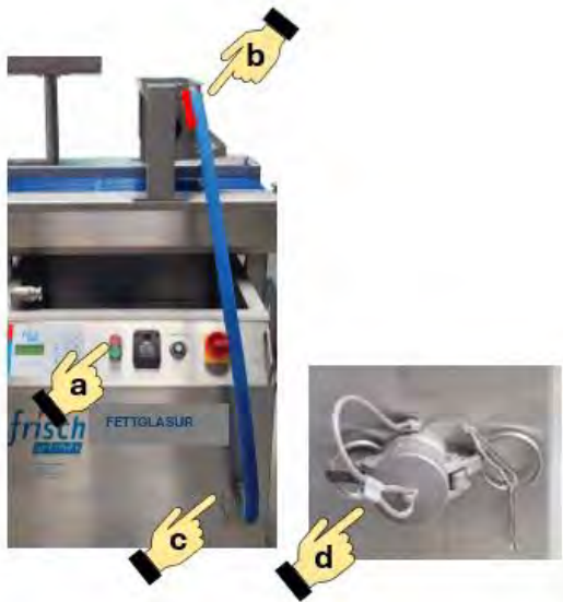
Figure 56: Close the material outlet
