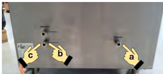
Figure 47: Flushing the HZ without a conductivity sensor
