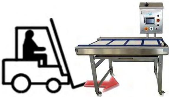
Figure 39: Lifting conveyor belts using a pallet truck or industrial truck
