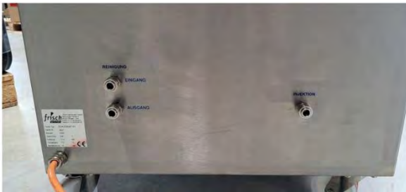
Figure 42: WIS water supply
