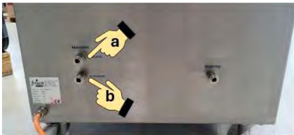
Figure 46: Flushing a heating machine with grease glaze
