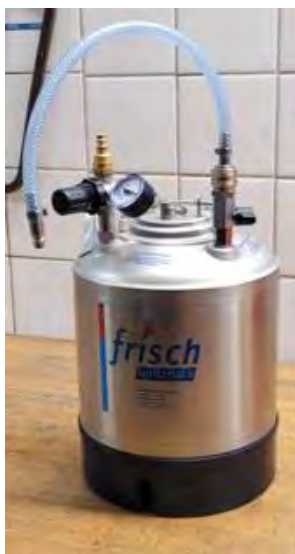
Figure 45: Oil pressure tank
